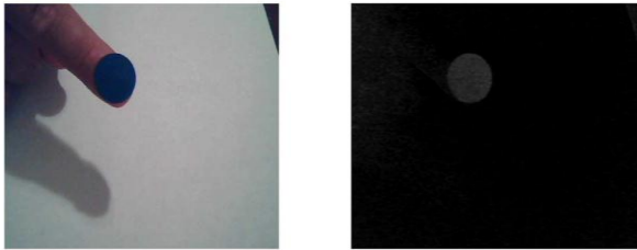
Figure 1. (a) Input image, (b) after using "imsubtract" and detect the blue color
