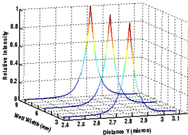
Figure 3(b) Near Field Intensity as a function of Well Width
