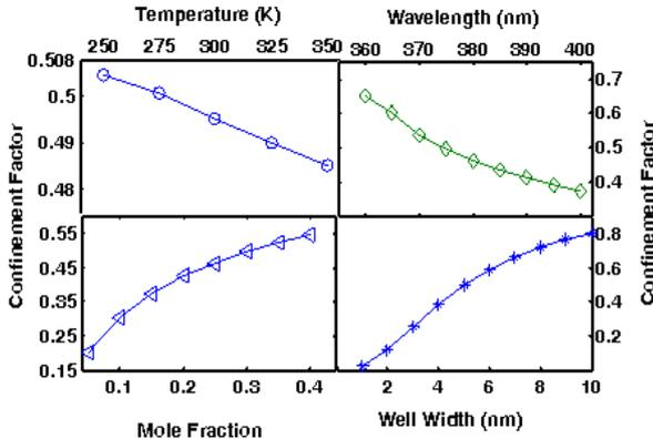
Figure 2 Dependence of confinement factor on various parameters.
