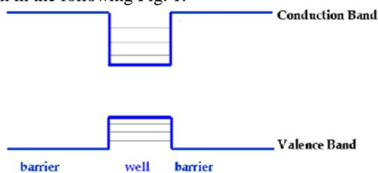
**Figure 1 III-V Nitride Single Quantum Well Schematic Structure**
