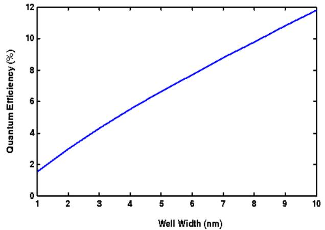
Figure 4(a) Quantum Efficiency variation with Well Width
