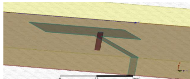
Fig.5 Designed Microstrip antenna with shorting pin(Zoomed View)
