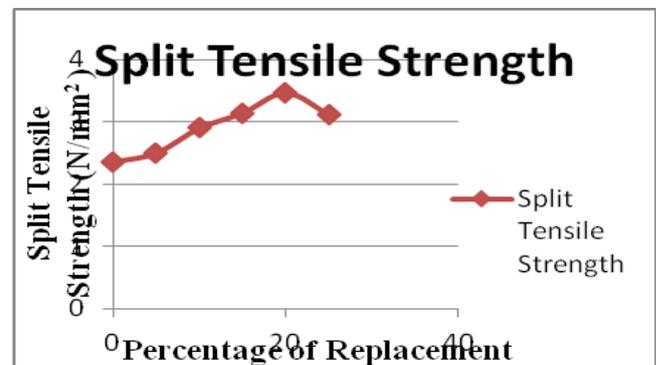
Fig.4.2 Variation of Split Tensile Strength
