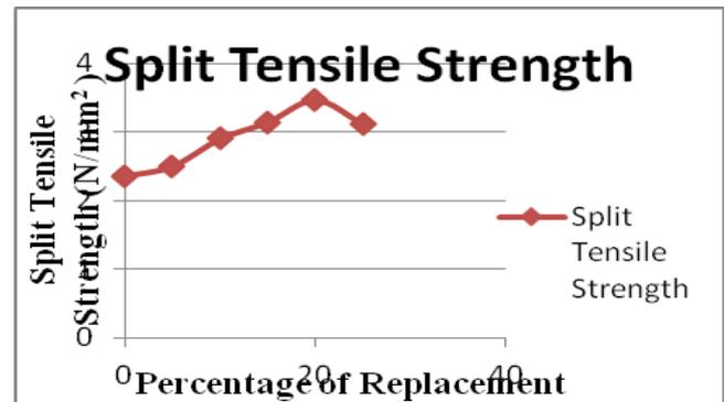
Fig.4.2 Variation of Split Tensile Strength
