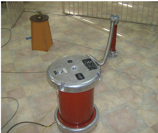
Figure (4): High voltage arrangement for determine break down test
