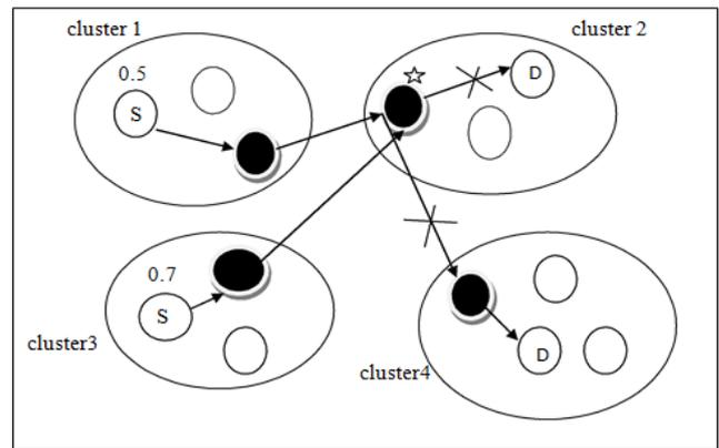
Figure 3.3: A network without synchronous nodes and packet collision
