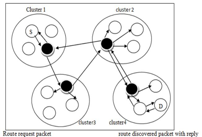
Figure 3.4: AODV routing protocol with route discovery
