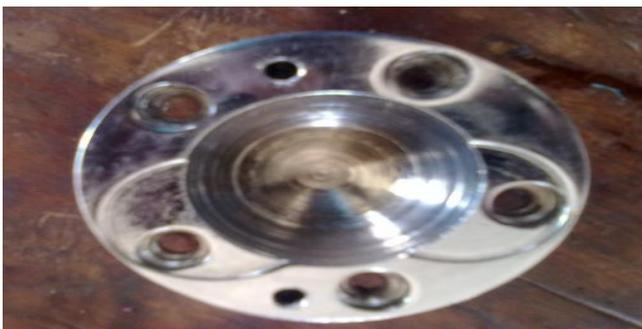
Fig 1: Air gap insulated Aluminum crown
