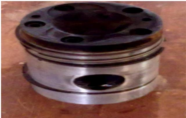
Fig 4: Photo of air gap Aluminum crown piston
