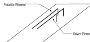
Fig.3 Dual inverted F antenna geometry
