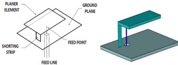
Fig.4 Basic layout of planar inverted F antenna.
