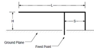
Fig.2 Inverted F antenna geometry
