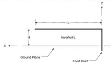
Fig.1 inverted L antenna geometry
