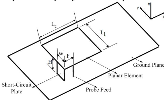
Fig.5 The structure of a PIFA with a finite ground plane
