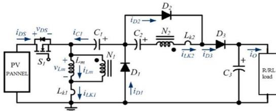
Fig.3 simplified model of proposed converter.
