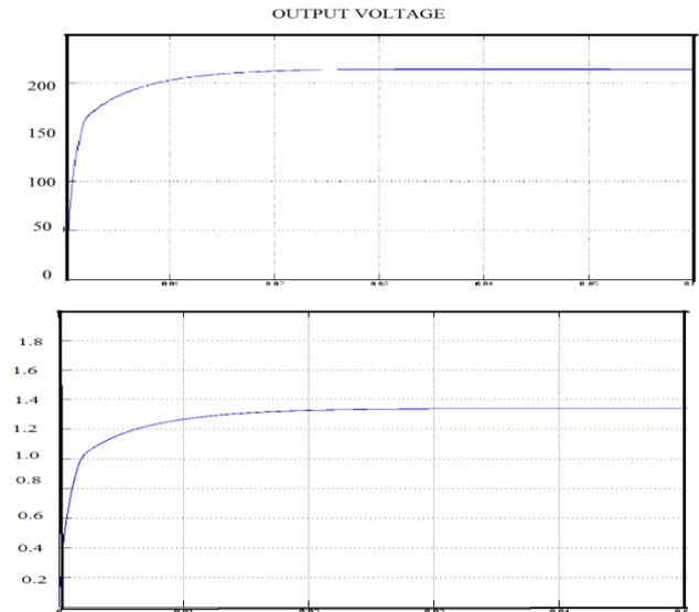
Fig.8.1 Output voltage and current for R load.
