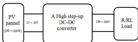
Fig.1 General configuration of DC module.
