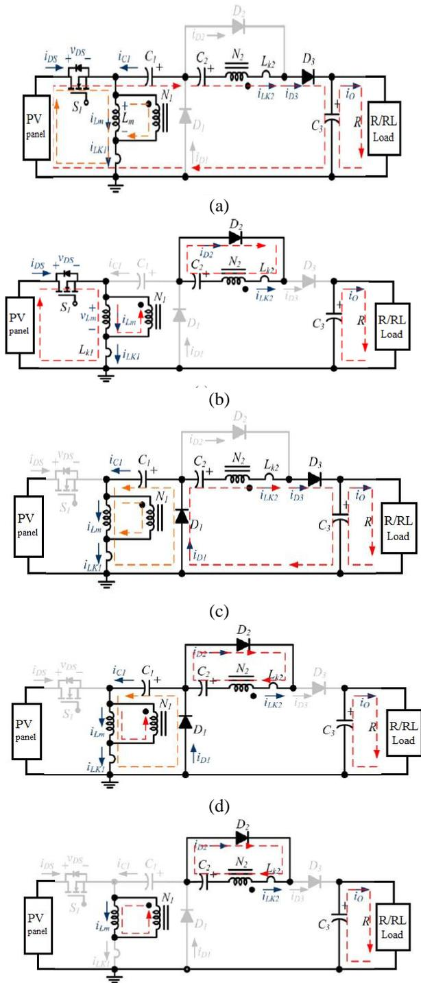
(e) Fig.5. During CCM operation, current flowing path in five modes operation (a) Mode I. (b) Mode II. (c) Mode III. (d) Mode IV. (e) Mode V.
