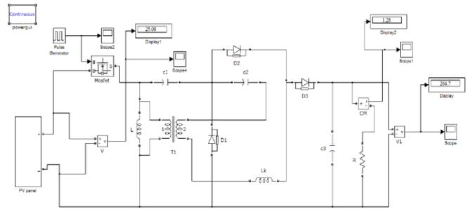
Fig.7.1 simulink model with R load.
