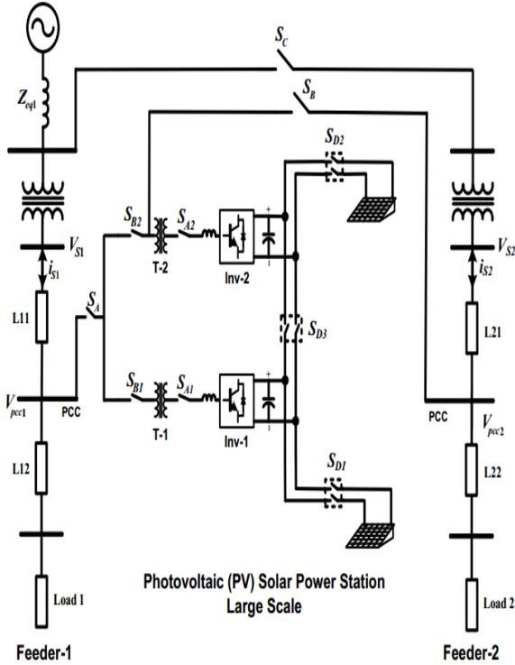
Fig. 1 Interline-PV (I-PV) power plant system configuration
