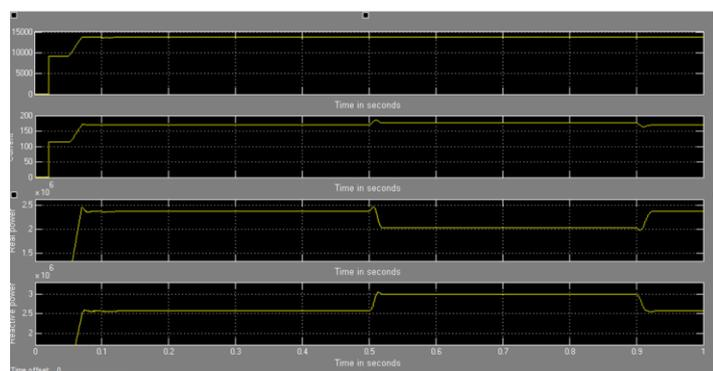
Fig. 7 Simulated output waveform for V, I, P and Q with PV plant in feeder 1.
