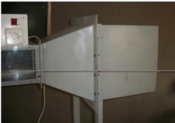
Fig 3: Showing the Stilling section
