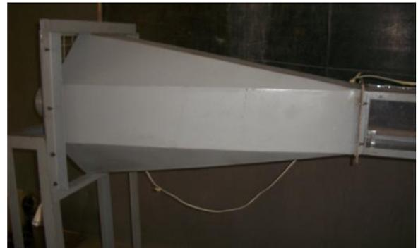
Fig 5: Showing the Contraction section
